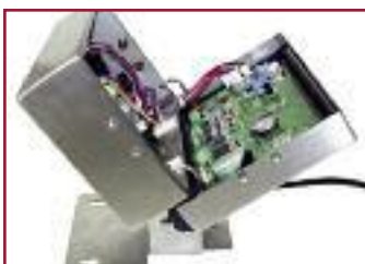
Internal hinge mechanism for ease of service
