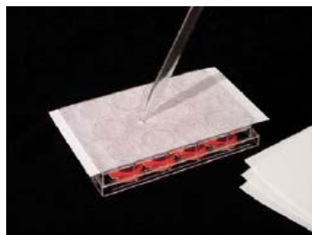
AeraSeal sealing films minimize cross-contamination, spillage and evaporation.
